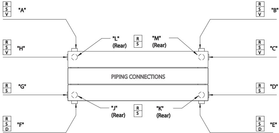
NOTE: ALL PR2, PR2F AND PR3F UNITS PROVIDED WITH SUPPLY CONNECTION ON FRONT HEADER AND RETURN CONNECTION ON REAR HEADER.
