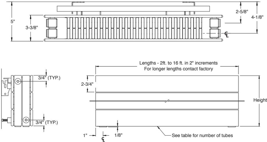
NOTE: ALL PR2F UNITS PROVIDED WITH SUPPLY CONNECTION ON FRONT HEADER AND RETURN CONNECTION ON REAR HEADER. UNIT SHOWN (AT RIGHT) WITH 1/2" NPT SIDE AND BOTTOM CONNECTIONS FOR DIMENSIONAL PURPOSES ONLY. REFER TO PIPE CONNECTION SHEET ON PAGE 17 FOR CONNECTION LOCATIONS AND SIZES OFFERED.
