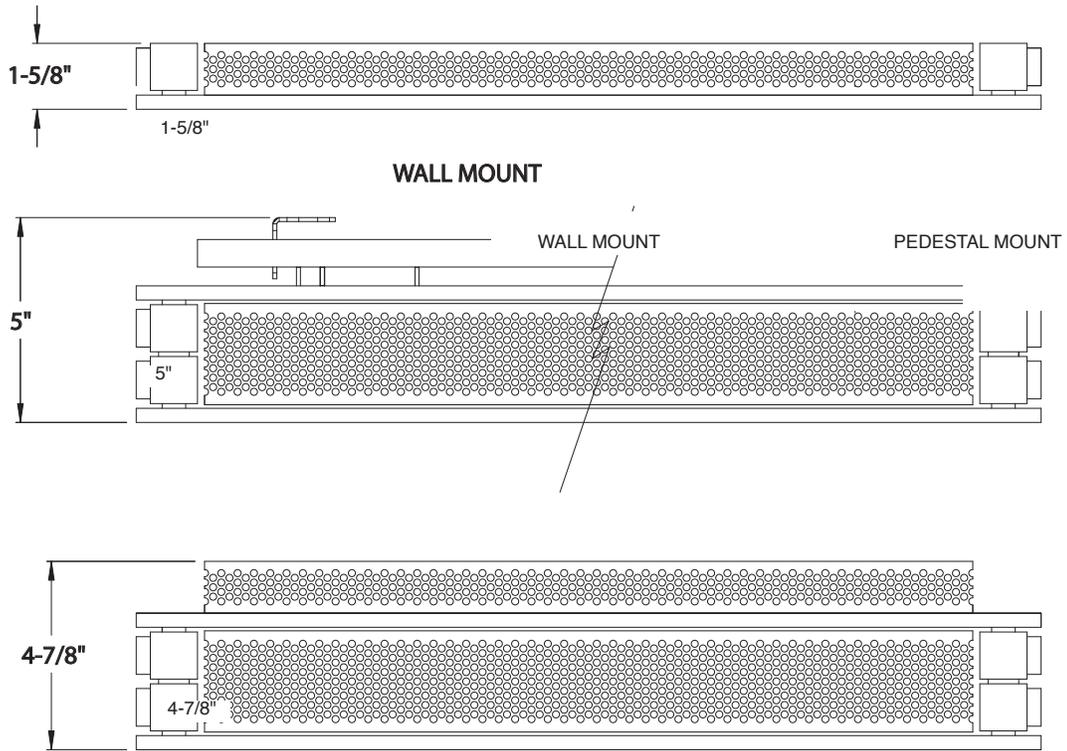
The 18-GA grille with 3/16" diameter holes on 1/4" staggered centerlines provides a pencil proof flat top to any standard panel. This allows for a more continuous look and prevents unwanted buildup between the fins. Grille is painted and finished with polyester epoxy powder to match the radiator. Adding the perforated grille may reduce output of some models.
