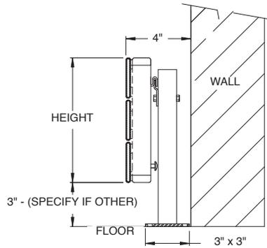
\* BRACKET IS FIELD INSTALLED (HARDWARE BY OTHERS) TO POST FOR STABILITY AND STRENGTH
