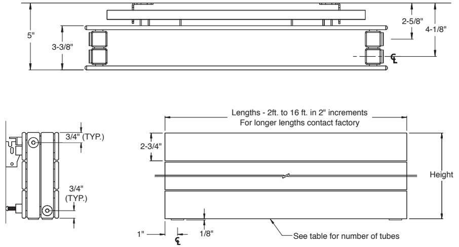
NOTE: ALL PR2 UNITS PROVIDED WITH SUPPLY CONNECTION ON FRONT HEADER AND RETURN CONNECTION ON REAR HEADER. UNIT SHOWN (AT LEFT) WITH 1/2" NPT SIDE AND BOTTOM CONNECTIONS FOR DIMENSIONAL PURPOSES ONLY. REFER TO PIPE CONNECTION SHEET ON PAGE 17 FOR CONNECTION LOCATIONS AND SIZES OFFERED.
