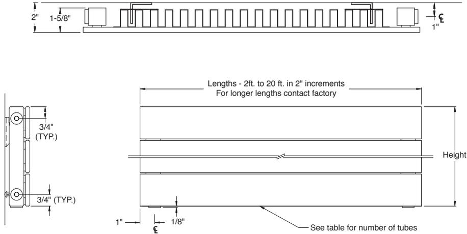
NOTE: UNIT SHOWN (AT RIGHT) WITH 1/2" NPT SIDE AND BOTTOM CONNECTIONS FOR DIMENSIONAL PURPOSES ONLY. REFER TO PIPE CONNECTION SHEET ON PAGE 17 FOR CONNECTION LOCATIONS AND SIZES OFFERED. NOT ALL HEIGHTS AVAILABLE WITH ALL LENGTHS.
