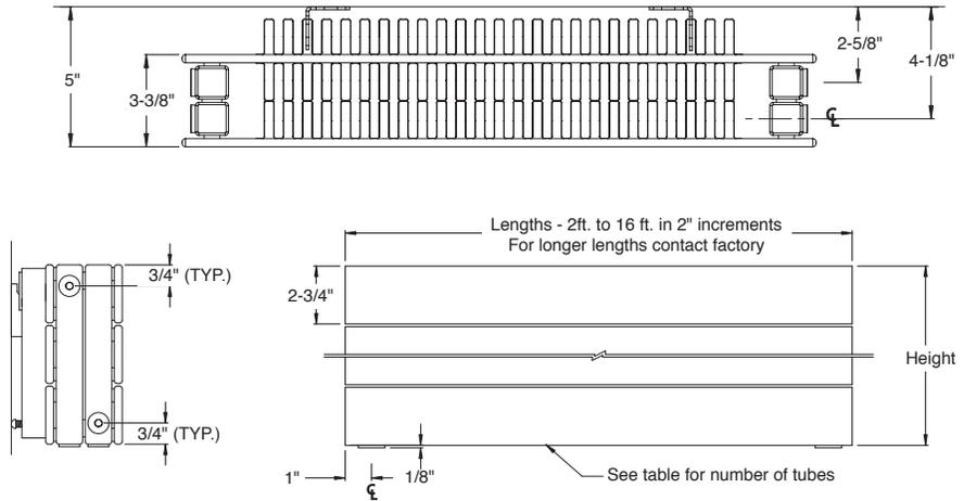
NOTE: ALL PR3F UNITS PROVIDED WITH SUPPLY CONNECTION ON FRONT HEADER AND RETURN CONNECTION ON REAR HEADER. UNIT SHOWN (AT LEFT) WITH 1/2" NPT SIDE AND BOTTOM CONNECTIONS FOR DIMENSIONAL PURPOSES ONLY. REFER TO PIPE CONNECTION SHEET ON PAGE 17 FOR CONNECTION LOCATIONS AND SIZES OFFERED.
