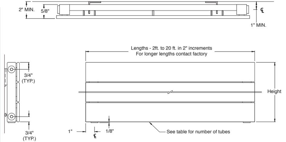
NOTE: UNIT SHOWN (AT LEFT) WITH 1/2" NPT SIDE AND BOTTOM CONNECTIONS FOR DIMENSIONAL PURPOSES ONLY. REFER TO PIPE CONNECTION SHEET ON PAGE 17 FOR CONNECTION LOCATIONS AND SIZES OFFERED. NOT ALL HEIGHTS AVAILABLE WITH ALL LENGTHS.
