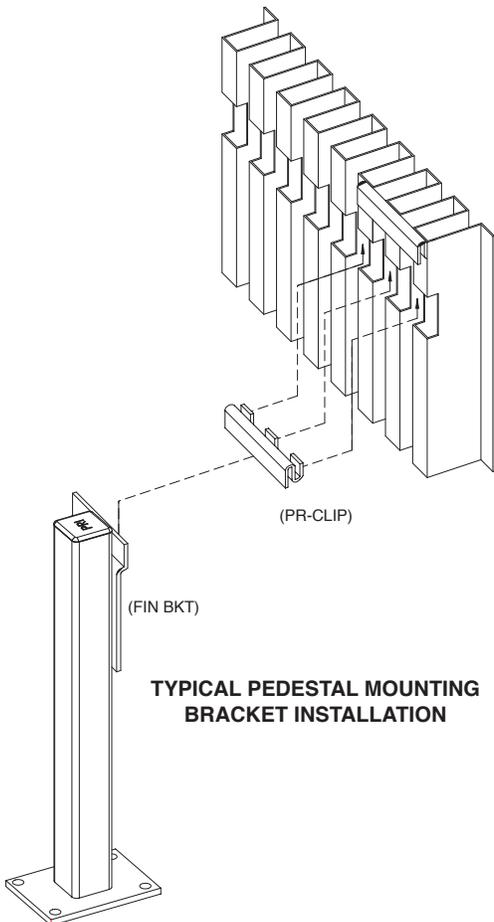
TYPICAL PEDESTAL MOUNTING BRACKET INSTALLATION
