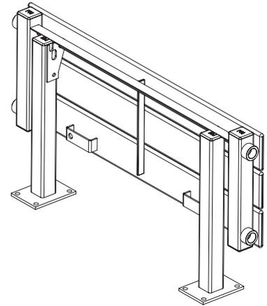
\* BRACKET IS FIELD INSTALLED (HARDWARE BY OTHERS) TO POST FOR STABILITY AND STRENGTH
