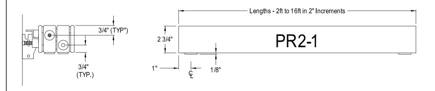
ALL PR2 UNITS PROVIDED WITH SUPPLY CONNECTION ON FRONT HEADER AND RETURN CONNECTION ON REAR HEADER.
