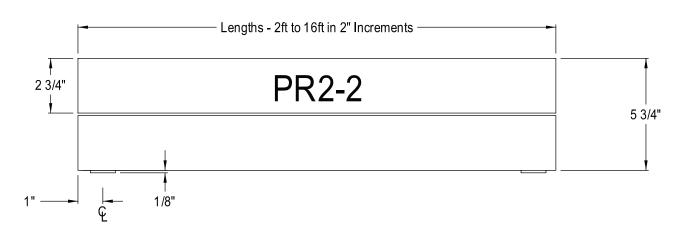
ALL PR2 UNITS PROVIDED WITH SUPPLY CONNECTION ON FRONT HEADER AND RETURN CONNECTION ON REAR HEADER.
