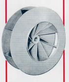
THE "XS" WHEEL is used where the air contains granular material which passes directly through the fan. The radial-type blades are more wear-resistant than those of the XB wheel. It is widely used in conveying systems for sawdust, chips, grain etc., with static pressures up to 16" in the standard design.
