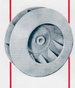
THE "XB" WHEEL has the highest efficiency of the four types shown. It is designed to handle air only or air containing fumes with a small quantity of fine dust. It is not recommended for handling coarse materials when they must pass through the fan. This wheel is utilized on applications such as hot gas, general supply or exhaust fan in many industrial processes and may also be used as an induced draft fan in power plants.
