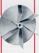
THE "XC" WHEEL is a modification of the XS with the same number of blades with with no shroud. It is used primarily as an exhauster handling stringy materials such as long shavings, rags etc., which may be fed directly into the fan inlet.
