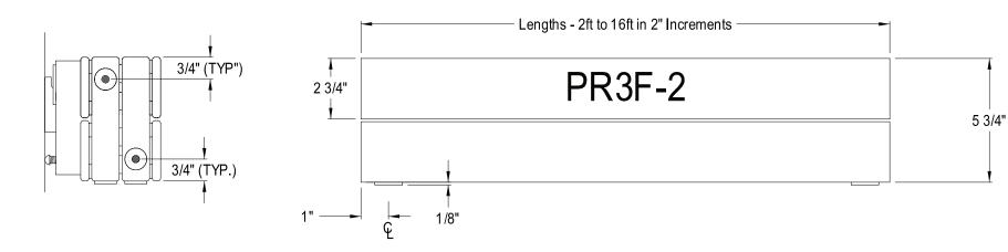
ALL PR3F UNITS PROVIDED WITH SUPPLY CONNECTION ON FRONT HEADER AND RETURN CONNECTION ON REAR HEADER.
